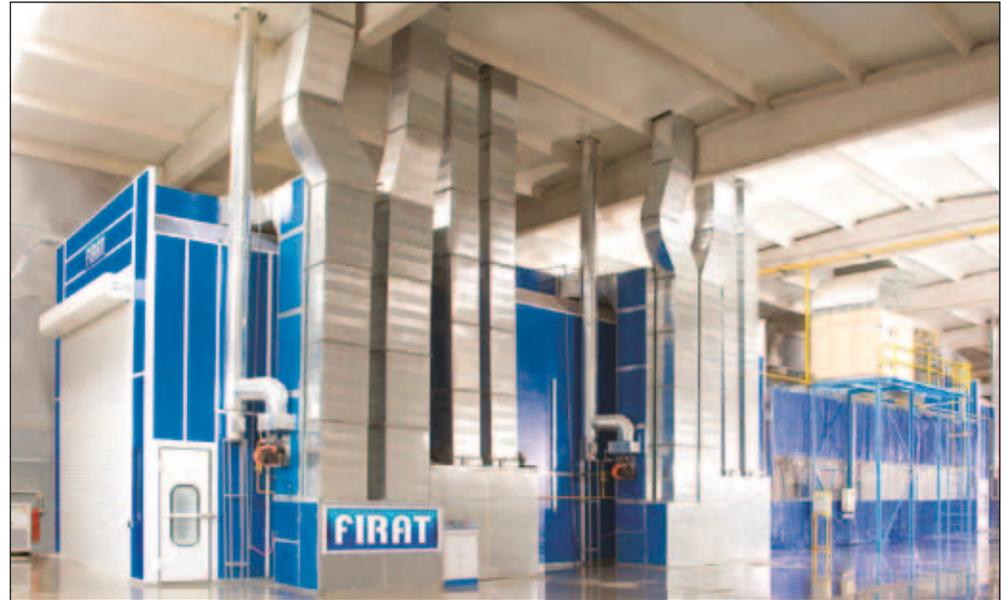
*Special Painting and Drying Booth, Special Preparation Station and Sandblasting Booth for Trailer*
