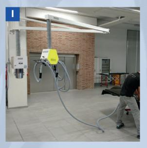
Articulated arms are the solution that allows to have at hand vacuum, air and power; or allows to clear the area to pursue different works and exploit completely the sizes at their disposal.
