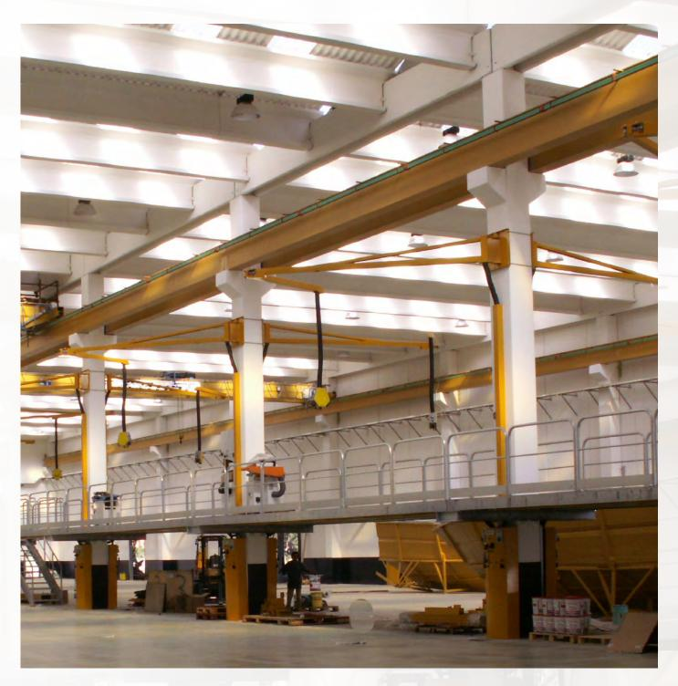
Articulated arms are available in three different measures B5 (5 m) e B6 (6 m) (if requested also 7 m). with this solution it's possible to remove the obstacle of electric cables, compressed air tubes and suction tubes.
