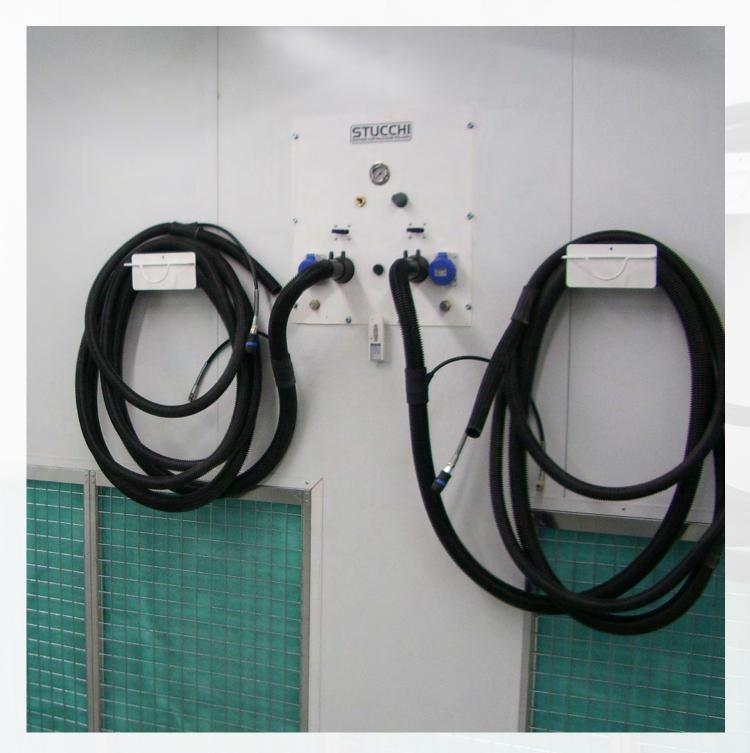
The automatic starter is with both electric and pneumatic tools. The suction system can be started using the remote start selector on the panel.
